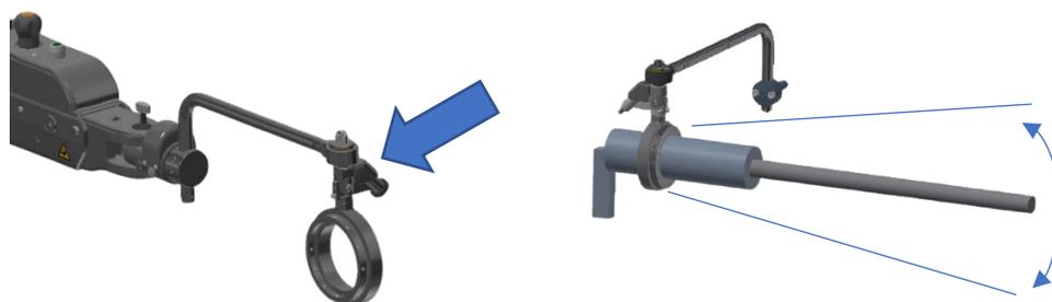
The dynamic balancer provides the angular buoyancy system, which allows it to absorb certain misalignments between the transversal axis of the tool and the nut or screw to be worked.
