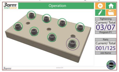
4. Bring the tool-arm assembly to the tightening position shown on the screen (flashing blue). When it is in the correct position the blue lights will flash with greater intensity. At this point the device will send the necessary signal to the device control to unblock the operation of the tool.
