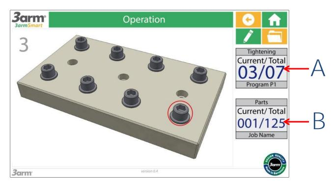
Tightening (Screw Number) (A): This box is for information. In the upper part, the current tightening position number is shown with respect to the number of total tightening positions defined for the current task or job. The numerator is actually a counter that will increase unitarily at the end of each tightening. Shown in the lower band, is the current tightening program. (Program P1) that the current tightening position corresponds to.
