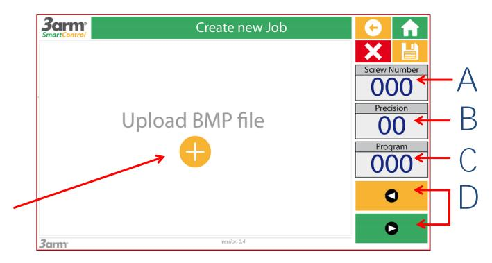
Upload BMP file: This area of the screen is reserved for embedding a representative image of the workpiece. The tightening positions will be defined in a layer above this.
