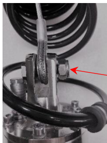
Fig. 21.45 The coupling (red arrow) should be loosened and the cable separated from the control unit.
