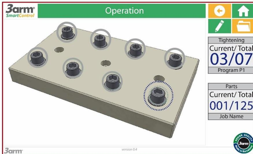
4. Bring the tool-arm assembly to the tightening position shown on the screen (flashing blue). When it is in the correct position the blue lights will flash with greater intensity. At this point the device will send the necessary signal to the device control of the tool to unblock the operation.
