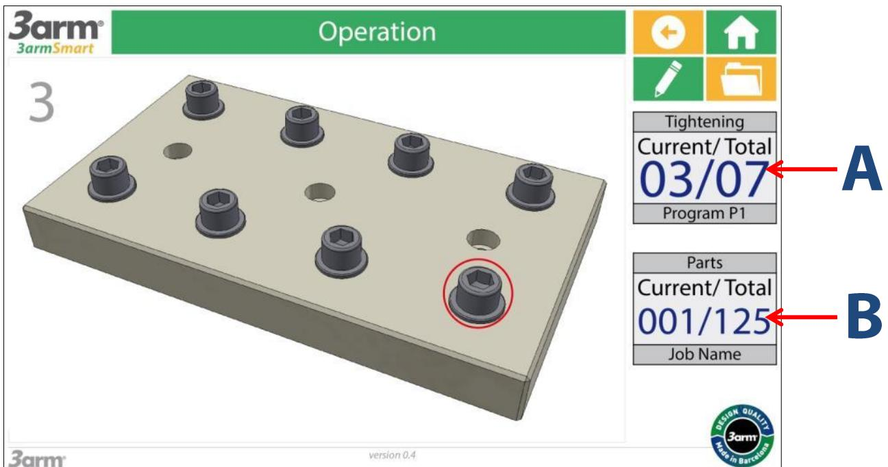
**Tightening (Screw Number) (A):** This box is for information. In the upper part, the current tightening position number is shown with respect to the number of total tightening positions defined for the current task or job. The numerator is actually a counter that will increase unitarily at the end of each tightening. Shown in the lower band, is the current tightening program. (Program P1) that the current tightening position corresponds to.
